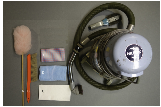
Fig. 1. Cleaning tools that were evaluated. (A) 100% pure lamb's wool duster. (B) Dusting brush. (C) Dust Bunny Reusable Nylon dusting cloth. (D) Microfiber cloth. (E) Chintz Duster, 100% cotton dusting cloth. (F) Nilfisk vacuum cleaner with HEPA filtration and brush head attachment.
