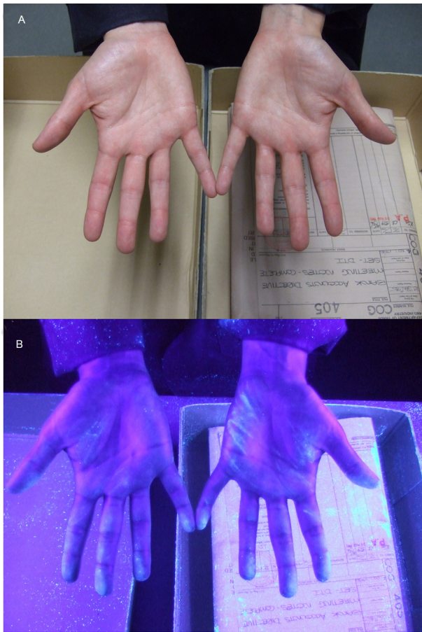
Fig. 3. Powder remaining on hands after 16 dust transfer sequences (A) as seen under office lighting and (B) as seen under UV lighting.
