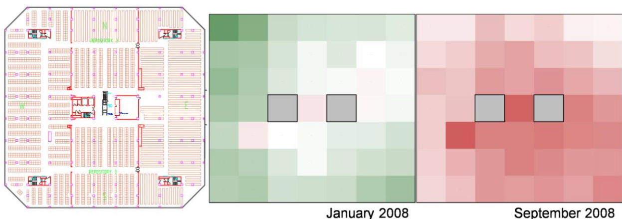
Figure 1. Example of permanence maps for 3rd Floor Q1. White is a permanence value of 1.33 while higher values become greener and lower values more red.
